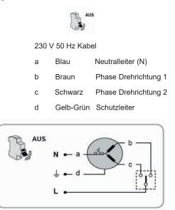
! Depending on the load capacity of the control unit and the drive variant used, several drives can be connected in parallel to one switching point.
